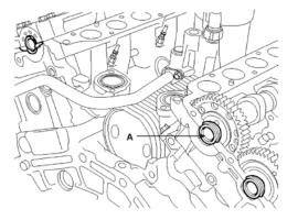
17. Install the camshaft bearing ladder (A) with the sequence and the torque below.
