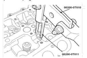
20. Remove the valve, valve spring and spring retainer
