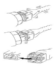
3. Slightly shake the connector and wiring harness vertically and horizontally.
