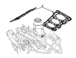
4. Place the cylinder head quietly in order not to damage the gasket with the bottom part of the end.
