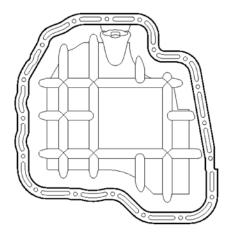
Liquid gasket: LOCTITE 5900 or equivalent
