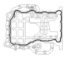
Liquid gasket: LOCTITE 5900 or equivalent
