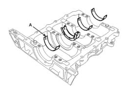
5. Place the bed plate on the cylinder block.
