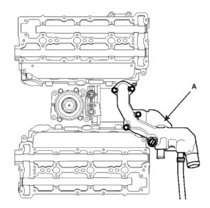
7. Remove the cylinder head cover(A).
