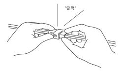
d. When a tester is used to check for continuity, or to measure voltage, always insert tester probe from wire harness side
