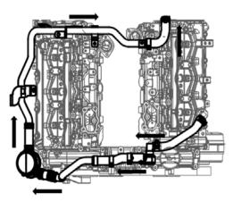
14. Remove the inlet lower manifold assembly(A).
