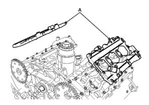
8. Remove the camshaft bearing ladder (A).
