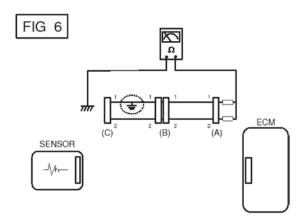
b. Disconnect connector (B), and measure the resistance between connector (A) and chassis ground, and between (B1) and chassis ground as shown in [FIG. 7].
