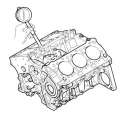
6. Check the cylinder bore size code on the cylinder block side face.
