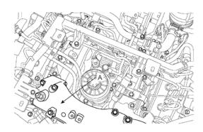
3. Disconnect the fuel pressure regulator valve & fuel temperature sensor connector (A).
