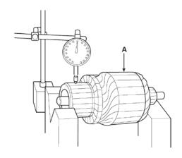
7. Check the mica depth(A). If the mica is too high(B), undercut the mica with a hacksaw blade to the proper depth. Cut away all the mica(C) between the commutator segments. The undercut should not be too shallow, too narrow, or v-shaped(D).
