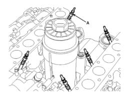
8. Install the water pipe and hose assembly(A).
