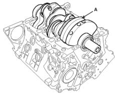
4. Aligning the bearing claw with the groove of the bedplate, push in the four lower bearings (A). Apply oil on the bearings at this moment.
