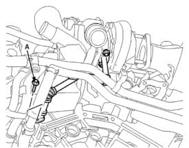
8. Remove the oil feed pipe and the blow-by hose(C).
