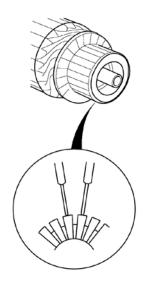
9. Check with an ohmmeter that no continuity exists between the commutator(A) and armature coil core(B), and between the commutator and armature shaft(C). If continuity exists, replace the armature.
