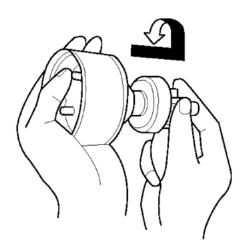
3. If the starter drive gear is worn or damaged, replace the overrunning clutch assembly. (the gear is not available separately)
