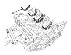
3. Place the crankshaft(A) on the cylinder block.
