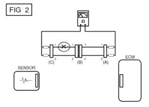
b. Disconnect connector (B), and measure for resistance between connector (C) and (B1) and between (B2) and (A) as shown in [FIG. 3]. In this case the measured resistance between connector (C) and (B1) is higher than 1<sup>MQ</sup> and the open circuit is between terminal 1 of connector (C) and terminal 1 of connector (B1)..
