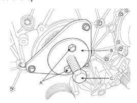
13. Push the pump shaft from the sprocket with rotating the main bolt (C) [SST No.: 00200-0T016] clockwise, and then remove the high pressure fuel pump from the engine. .
