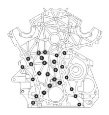
3. Install the water pump(A) with a new gasket.
