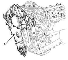
13. Remove the hydraulic tensioner(A).
