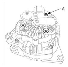
2. Remove the alternator cover(A) using a screw Drive(B)
