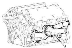
Installation is in the reverse order of removal. Water Outlet Duct and Fitting
