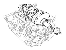
3. Inspect the crankshaft main journals and pin journals. Using a micrometer, measure the diameter of each main journal and pin journal.
