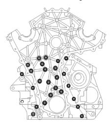
20. Remove the chain case assembly(C).
