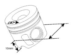
3. Calculate the difference between the cylinders bore inner diameter and the piston outer diameter.
