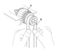
5. Check the commutator diameter. If the diameter is below the service limit, replace the armature.
