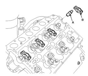
1) After you removing it, HLA shall be held upright so that oil in it should not spill and be assured that dust does not adhere to it.
