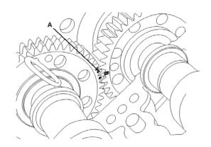
When installing the RH exhaust camshaft always check the location of TDC(top dead center) mark on the shaft.
