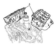
17.Remove the cylinder head gasket(A)
