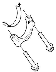
13.Install the piston and connecting rod assembly.
