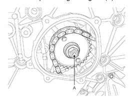
11. Install the fixing plate (A) [SST No.: 00200-0T016] on the timing case. .
