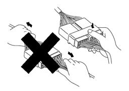
b. When removing the connector with a lock, press or pull locking lever.
