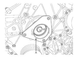
12. Install the supporter (B) [SST No.: 00200-0T016] on the sprocket with the bolts (A) [SST No.: 00200-0T016].
