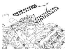
2. Install the inlet lower manifold assembly(A).
