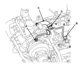
9. After removing the rest turbocharger mounting nuts(A), take off the turbocharger by lifting up.
