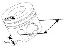
3. According to the measured outer diameter, calculate the new bore size.
