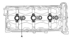
16. Install the sealing caps (A) with applying sealant LOCTITE 5902/5900 or equivalent) on the grooves (4 places) at the circumference.
