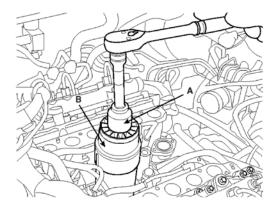
2. Remove the oil filter paper (A) and its O-ring (B) from its cap
