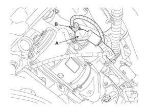
2. Remove the starter by loosening the starter mounting bolts(A).
