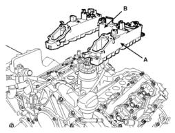
17. Remove the inlet manifold gaskets(A).
