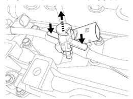
2. Seize the return line on both sides of the plug, and then disconnect the plug upward from the injector nipple
