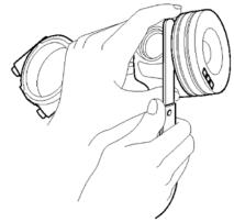
If the clearance is out of the specification above replace the piston.
