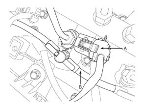
3. Disconnect the injector return line (B).
