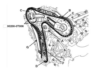
10.Install the hydraulic tensioner(A).
