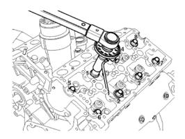
6. Install the timing chain case bracket (A). Tighten the vertical-direction bolts slightly first and then the horizontal-direction ones and the vertical-direction ones with the specified torque below.
