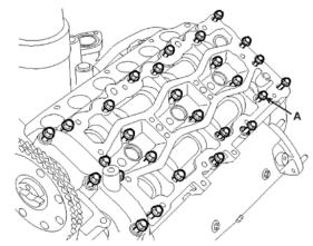
9. Remove the sealing cap (A) from the cylinder head assembly.
