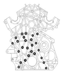
4. Apply liquid gasket on the upper oil pan assembly shown as below.
