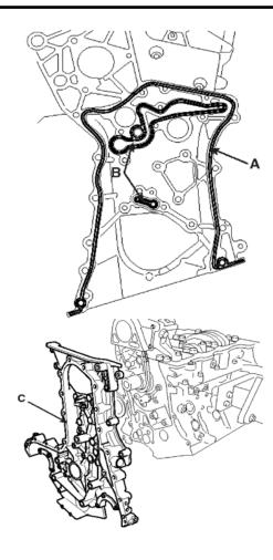
3. Tighten the mounting bolts of the chain case with the specified torque below.
