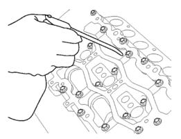
19. Install the cylinder head cover (A) with the sequence and the torque below.
