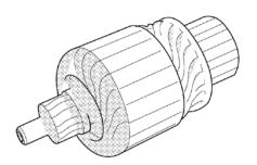
4. Check the commutator(A) surface. If the surface is dirty or burnt, resurface with emery cloth or a lathe within the following specifications, or recondition with #500 or #600 sandpaper(B).
