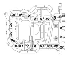
6. Apply liquid gasket on the lower oil pan assembly shown as below.
