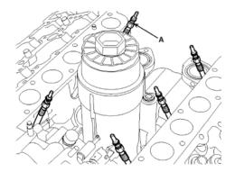
14.Remove the timing chain case bracket(A).
