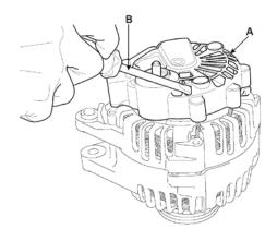
Loosen the mounting bolts (A) and disconnect the brush holder assembly(B) 4. Remove the slip ring guide(A)
