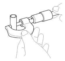
Measure the piston pin-to-piston clearance.
