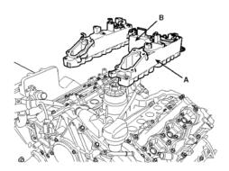
3. Install the blow-by gas recirculation system such as the oil separator pipes and hoses.
